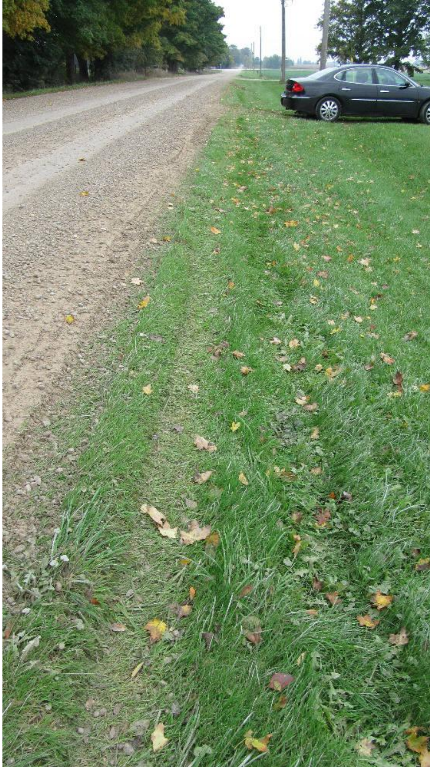
Figure 23: View, looking west, at the tire marks near the edge of the grass that can be firmly attributed to the pre-crash motion of the school bus.
