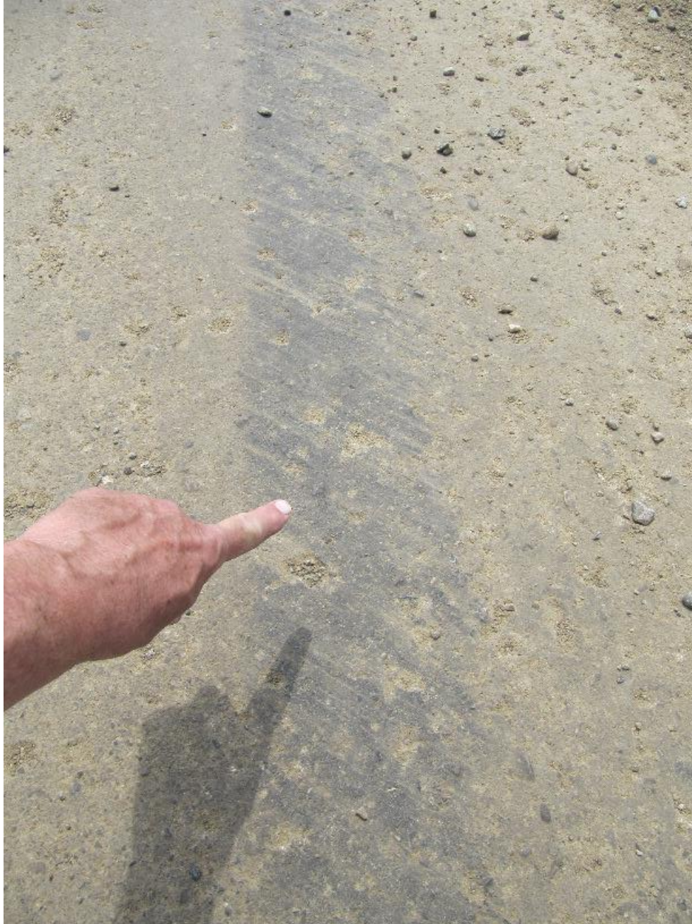
Figure 17: Yaw marks indicative of a vehicle's loss-of-control rotation can be detected on the packed portion of the surface. As typical, the angle of the striations within the mark will reveal any indication of braking or acceleration.
