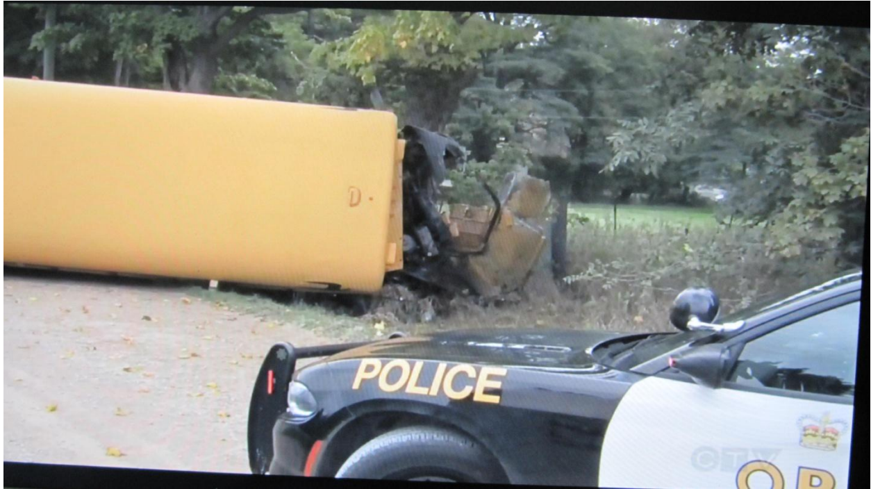
Figure 10: View showing the substantial frontal crush to the bus as a result of the tree impact.
